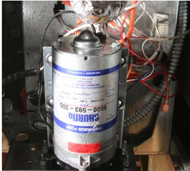
Figure 9: Position the pump on the provided bracket.
