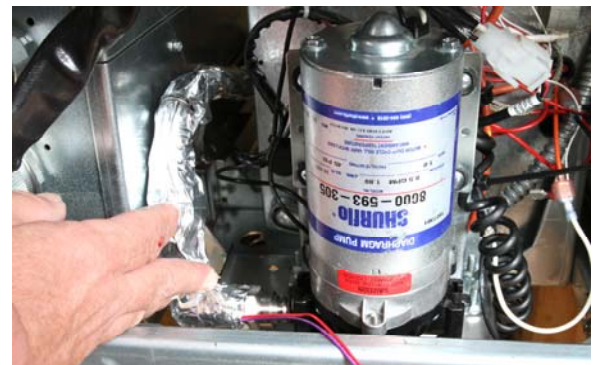
Figure 21: Route the wrapped flex line to the pump inlet side.
