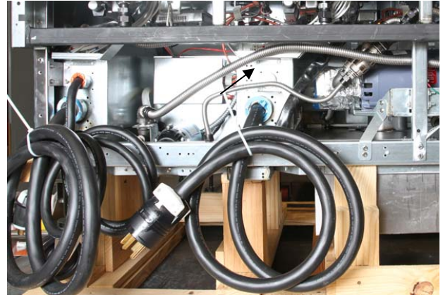
Figure 20: Remove element wire protective shields..
