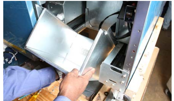
Figure 15: The heated JIB platform must enter the JIB cabinet at a steep angle.
