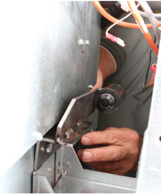
Figure 7: Positioning female oil pickup on fryer channel. It will be necessary to lift the contactor box to position nuts on the 1/4 x 20 bolts securing the pickup. May not be necessary in newer fryers.
