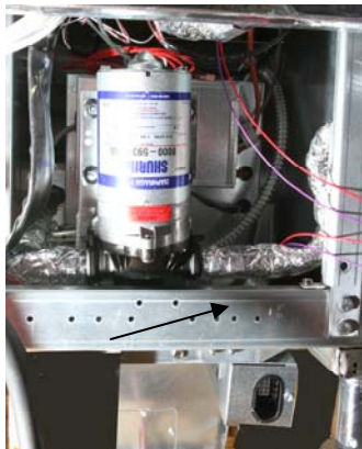
Figure 16: Mount the thermostat housing under the ATO pump bracket.
