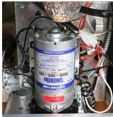
Figure 17: Route the heater controller wire over the pump and to the right.
