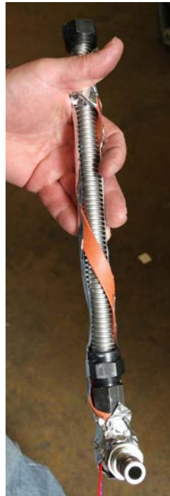
Figure 22: Wrap the provided, larger diameter, inlet and outlet flex lines with heater tape. Ensure the wire leads exit near the junction box position.
